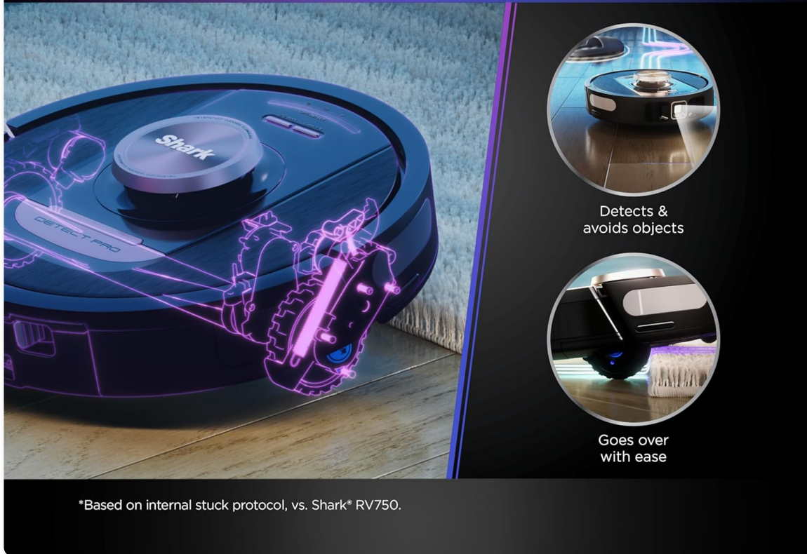
Figure 6: An illustration of NeverStuck Technology, showing the robot's internal mechanisms lifting its body to clear obstacles and thick carpets.
