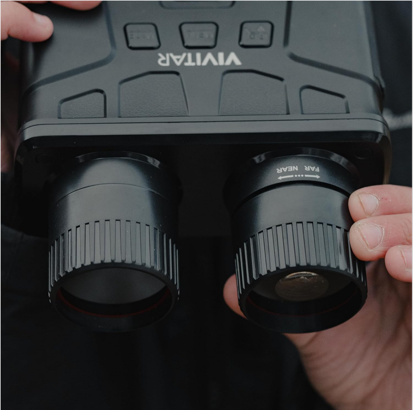
A user's hands demonstrating the adjustment of the focus ring on the binoculars' objective lens.
