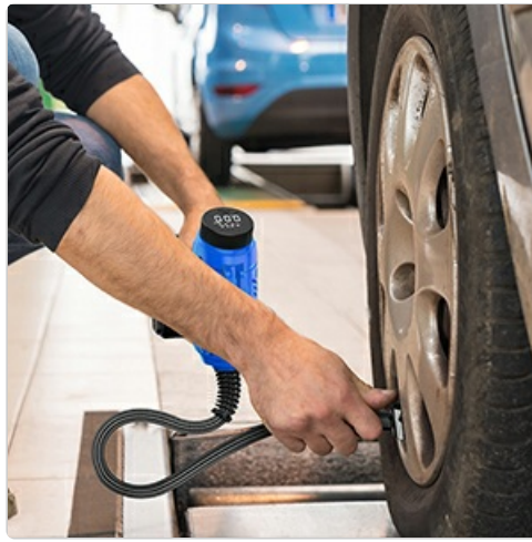
Image: A person attaching the inflator's hose to a car tire valve, illustrating the first step of operation.
