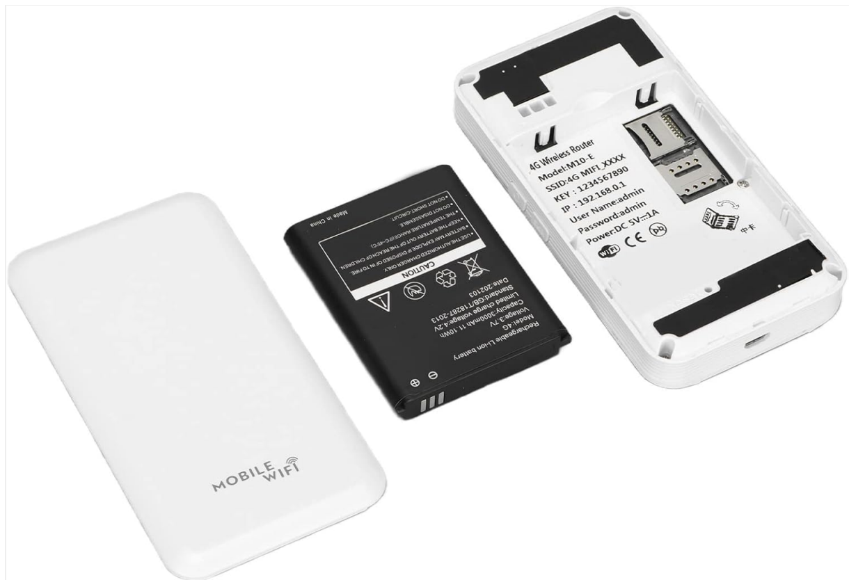
Image 3.1: Internal view of the Jectse M10-3, showing the battery compartment and the SIM card slot for network connectivity. Note the default Wi-Fi credentials printed on the label: IP: 192.168.0.1, User Name: admin, Password: admin.
