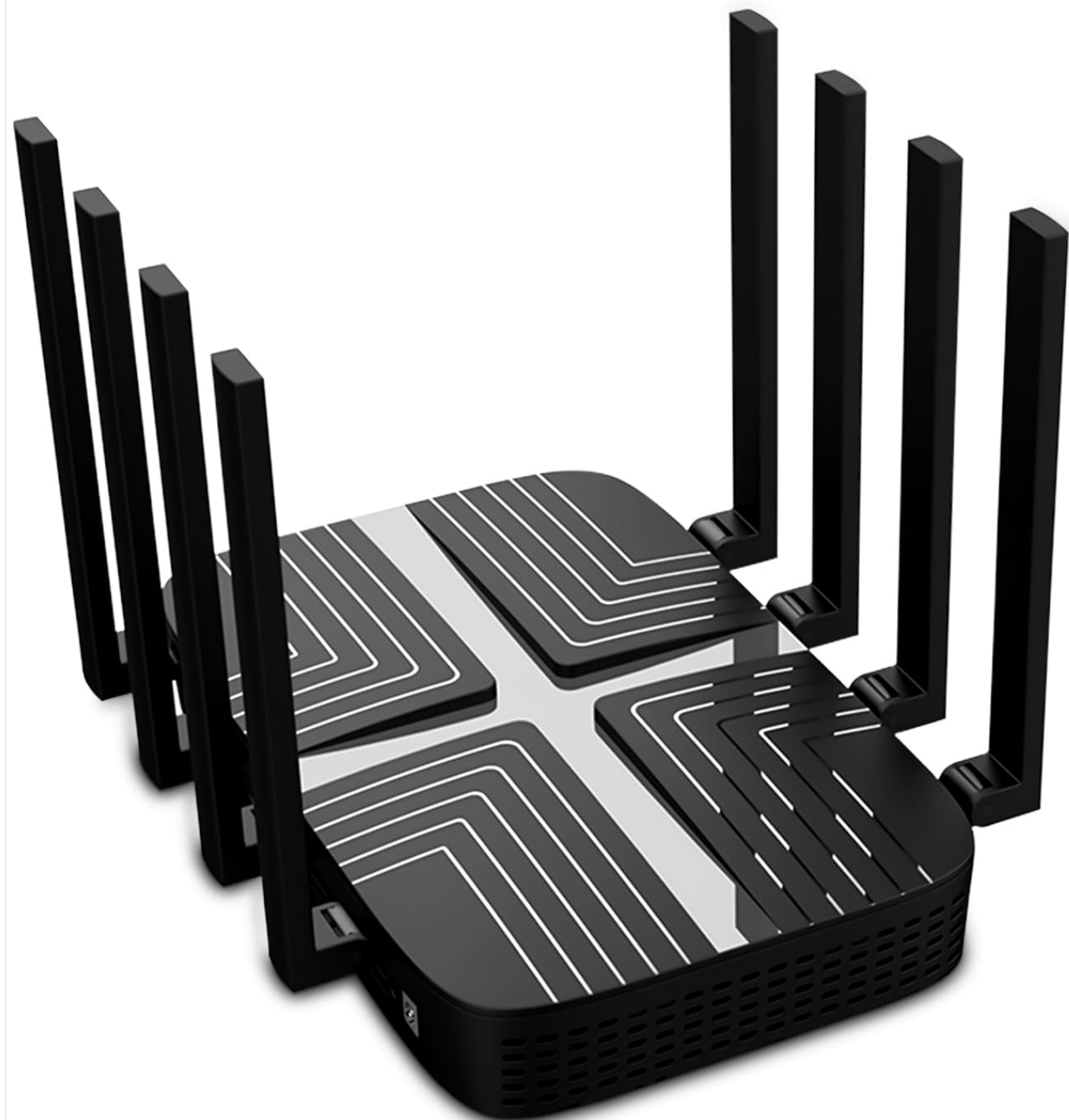
Figure 1: Wiflyer AX3000 Cat9 4G LTE Router (Model Z8102-M2-S) with multiple antennas.
