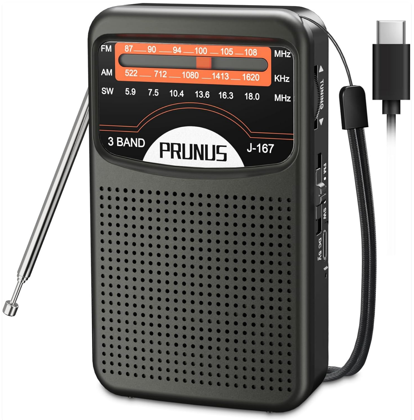
Image 1.1: Front view of the PRUNUS J-167 Portable Radio, showing the frequency display, speaker, and extended telescopic antenna.
