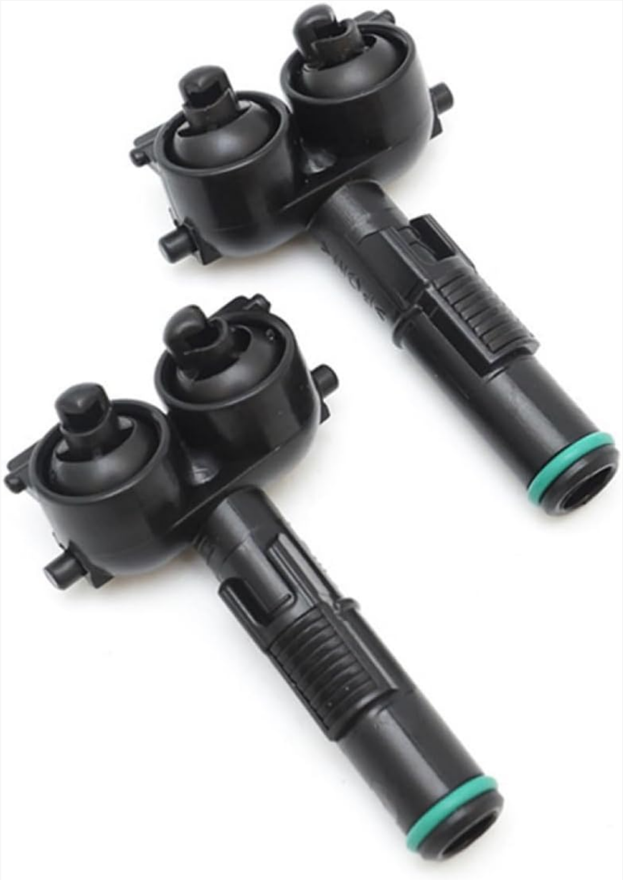
Figure 5.1: Two headlight washer nozzles, illustrating the slight difference between left and right variants. Ensure the correct part (Right side, BP4K-51-8G1B) is used for installation.
