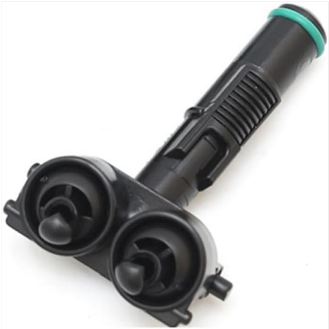
Figure 2.2: Angled view of the headlight washer nozzle, highlighting the textured grip area and the connection point.
