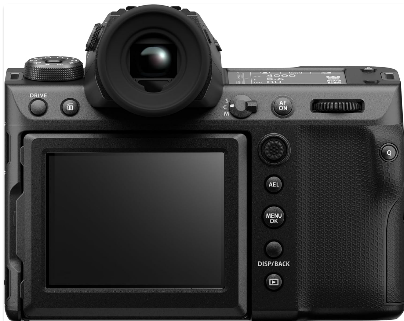
Figure 3.1: Rear view of the camera, highlighting the LCD screen, EVF, and control layout.
