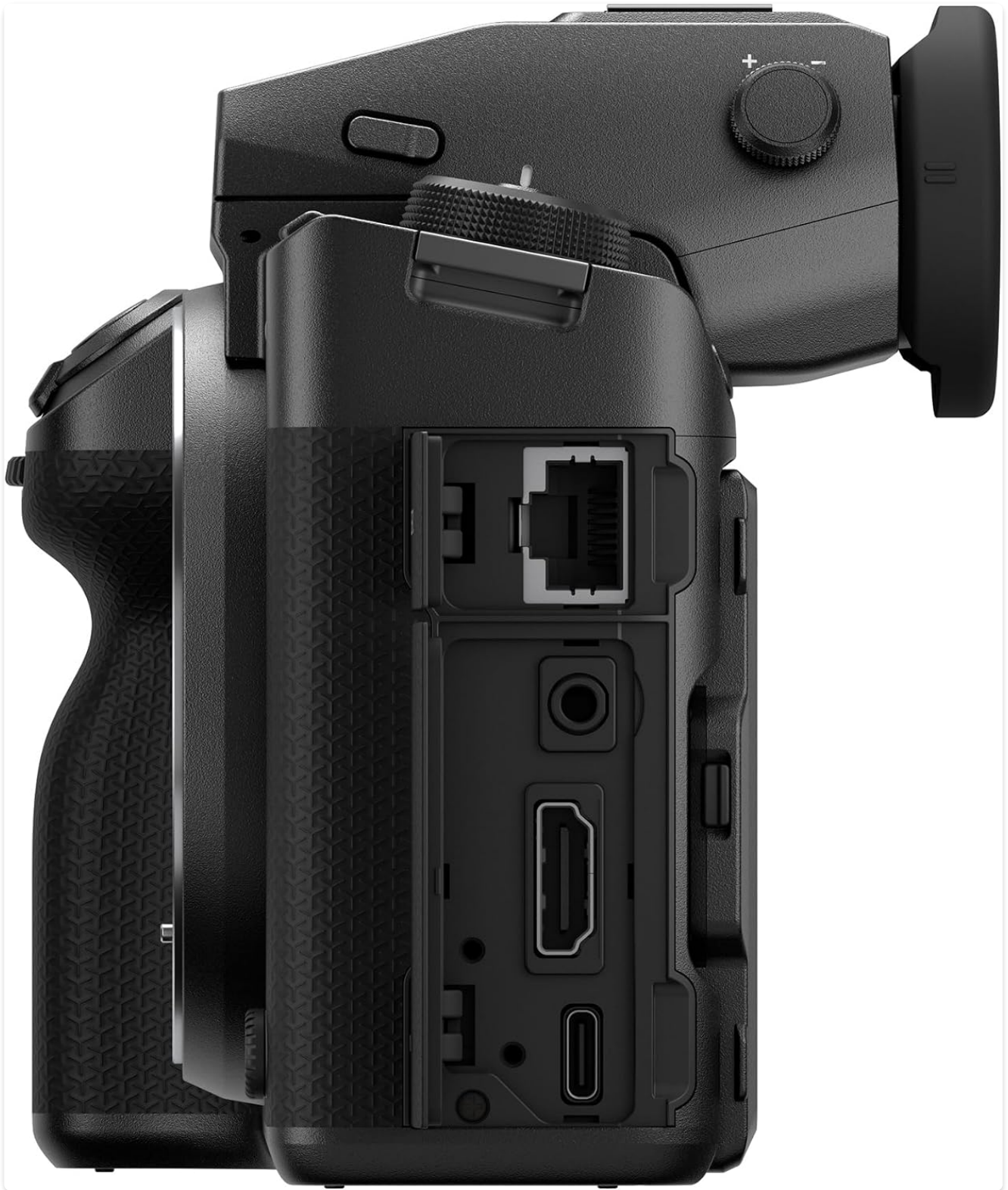
Figure 3.9: Side view of the camera with port covers open, showing various connectivity options.
