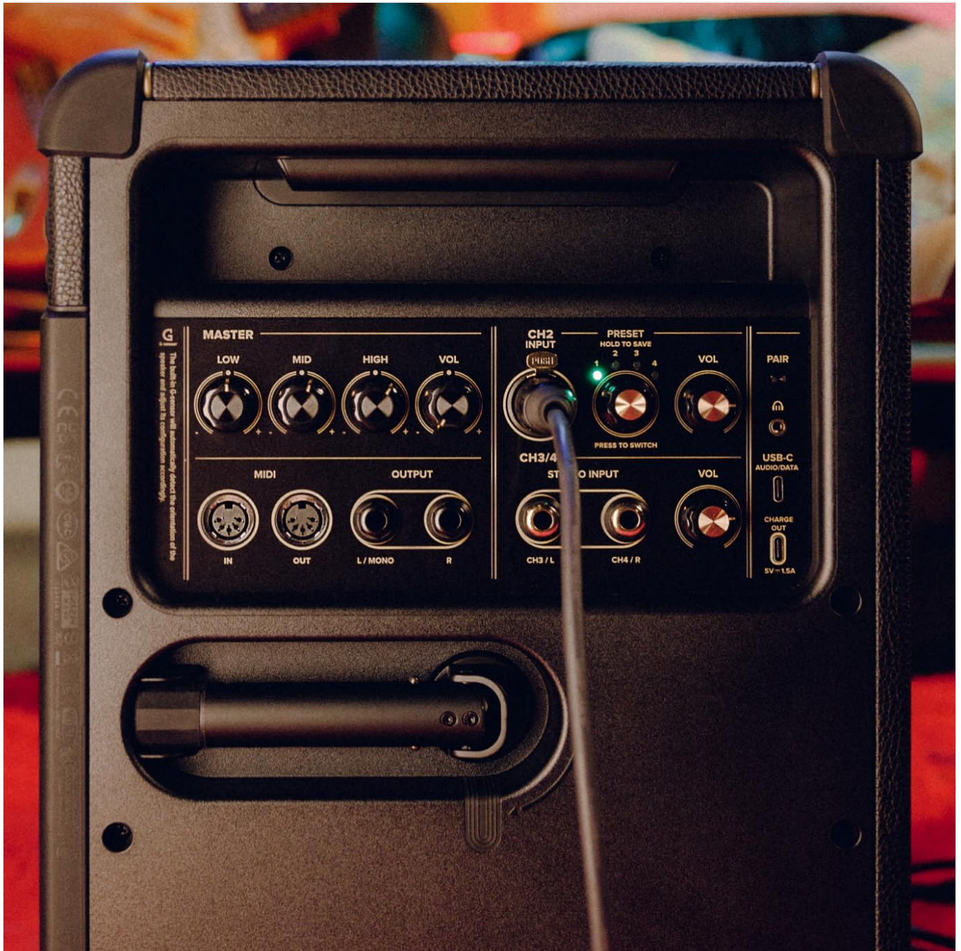
Figure 3: Rear panel connections for the Spark Live.
