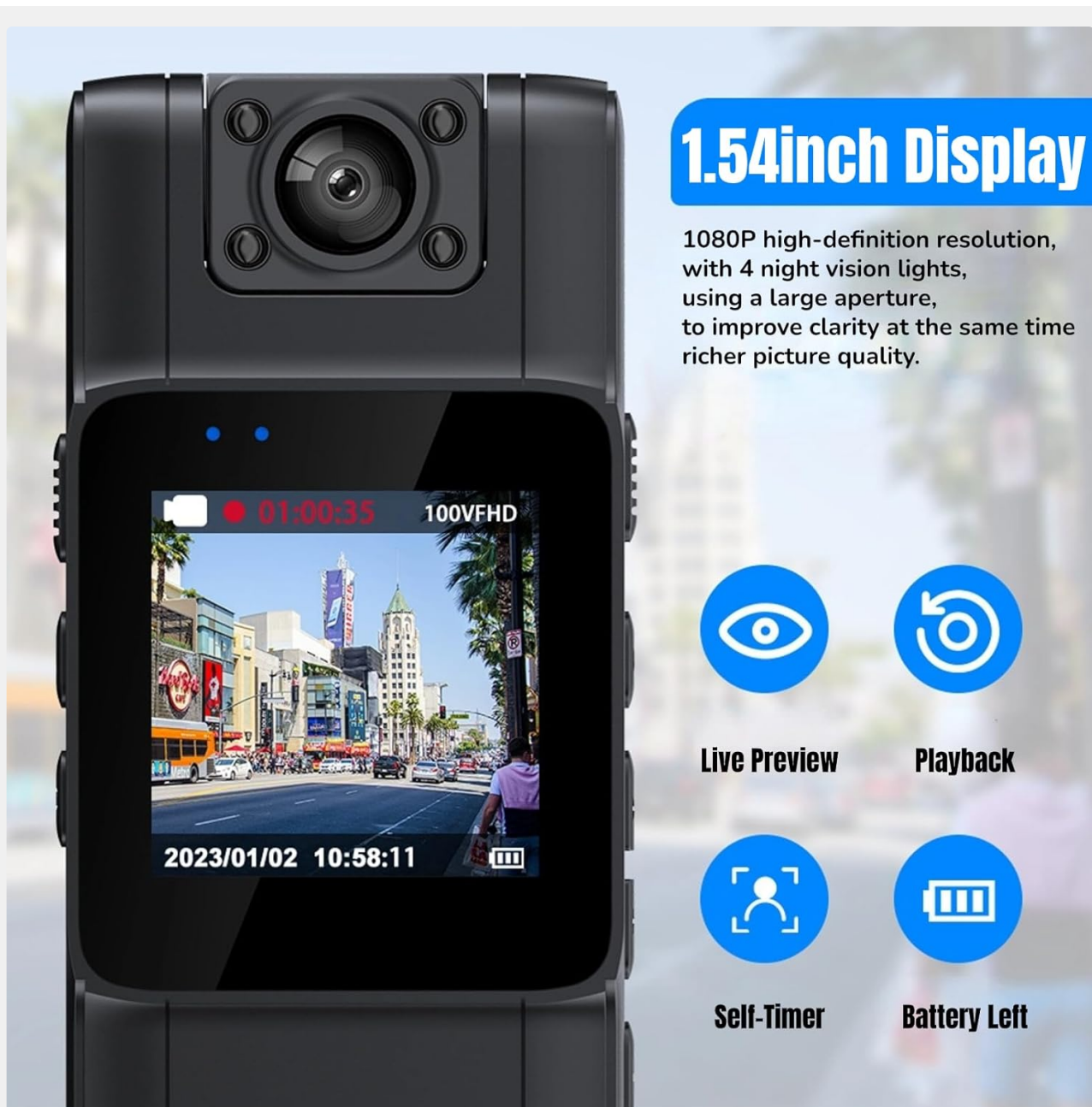
Figure 1.4: The 1.54-inch display, providing live preview, playback, self-timer options, and battery status.
