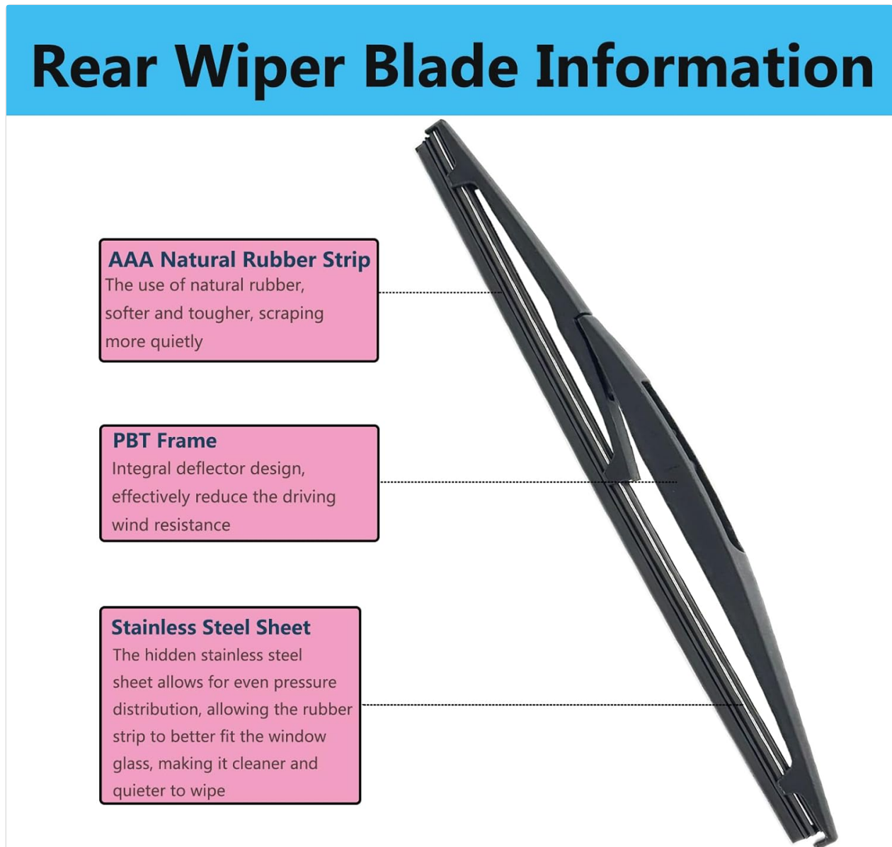
Image 2.1: Detailed view of the wiper blade components.
