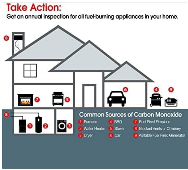
Image 2.1: Diagram illustrating common sources of carbon monoxide within a household, including furnaces, water heaters, dryers, stoves, BBQs, cars, fuel-fired fireplaces, blocked vents, and portable fuel generators. It emphasizes the need for annual inspections of fuel-burning appliances.
