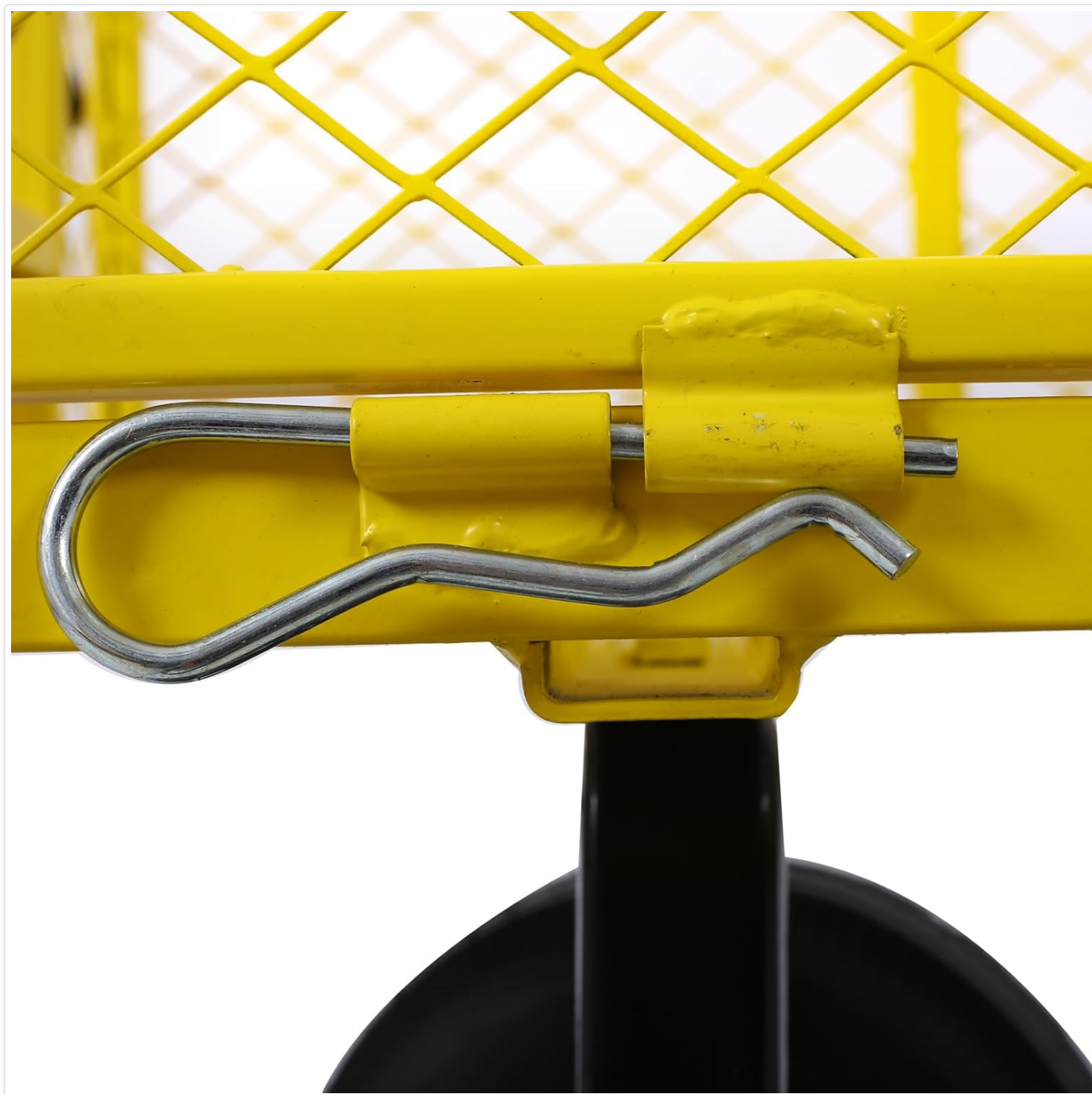
Image: Detail of the securing pin, which must be fully inserted to hold the side panels in place.
