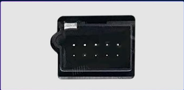
A 10 pin LVDS post at the rear of the unit
