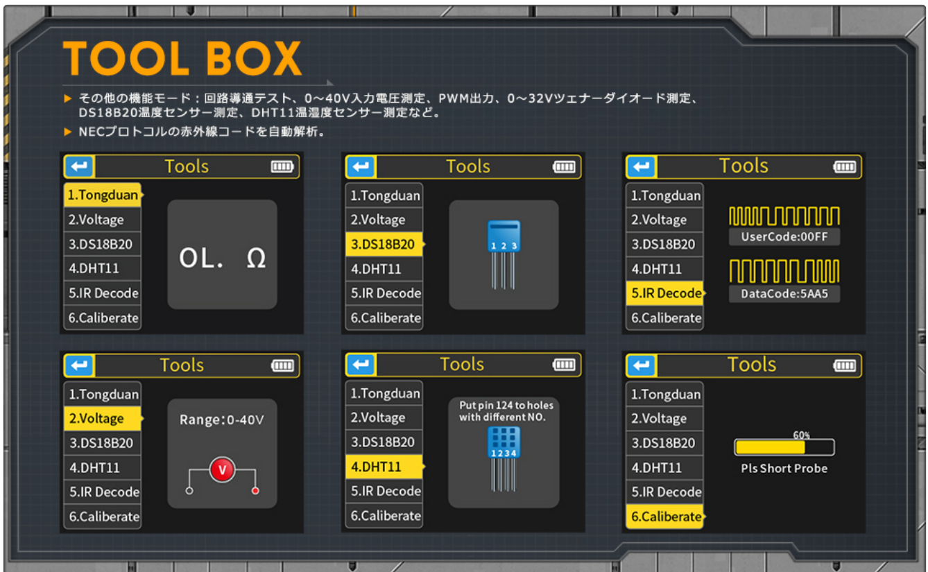
Figure 5.1: The Tool Box menu, providing access to advanced diagnostic and measurement utilities.
