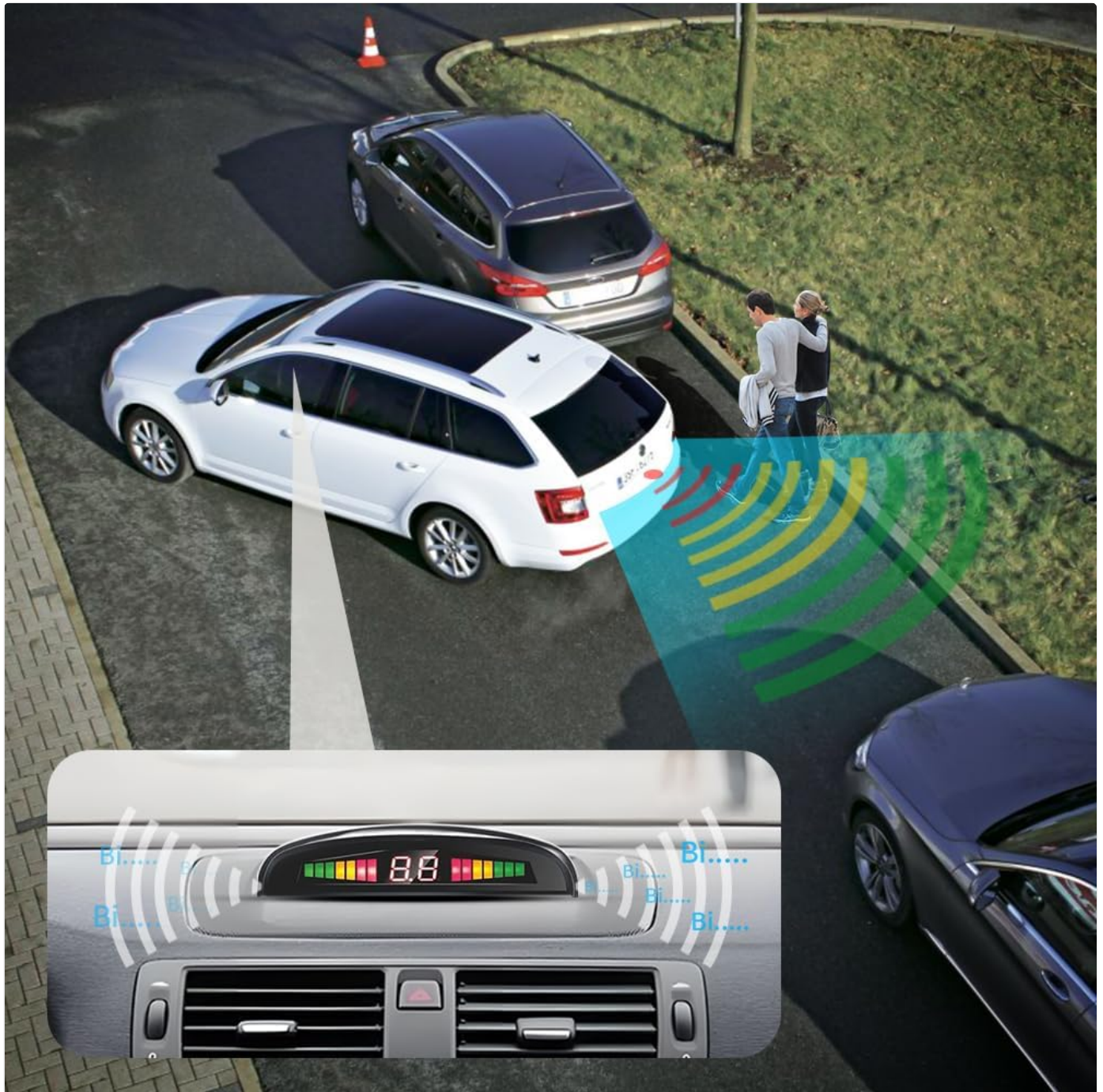
Figure 5.1: An illustration of the parking assist system in action, showing a car reversing, sensors detecting an object, and the LED display providing visual feedback to the driver.
