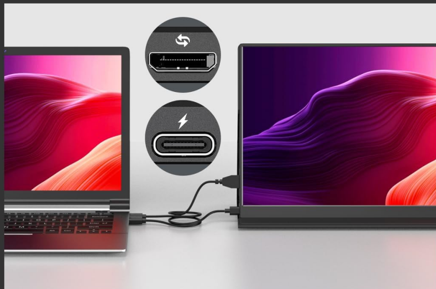
Figure 3.3: Dual Cable Connection (HDMI + Power)
