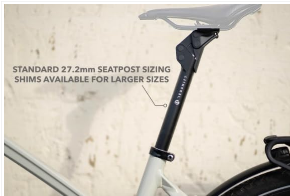
Image: The ShockStop seatpost on a bike, illustrating the standard 27.2mm sizing and the availability of shims for larger seat tube diameters.
