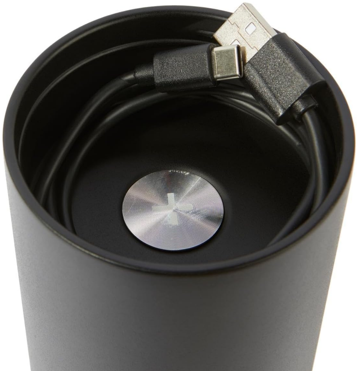
Figure 3: The convenient storage compartment for the USB-C charging cable within the power bank base.
