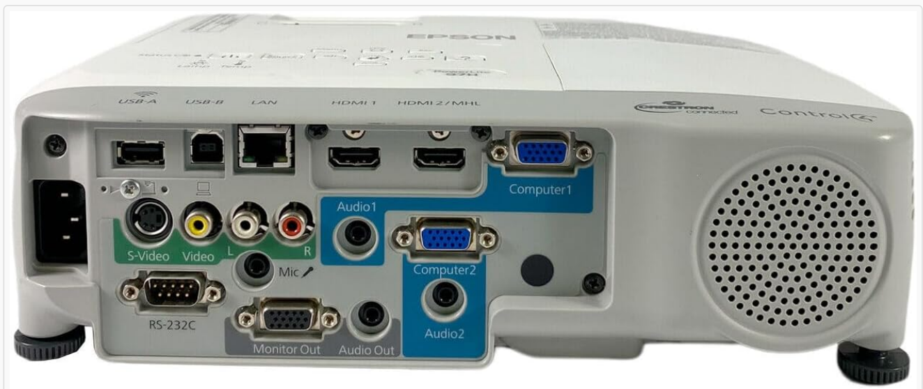
Figure 1: Rear panel of the Epson PowerLite 97H Projector showing various input and output ports.
