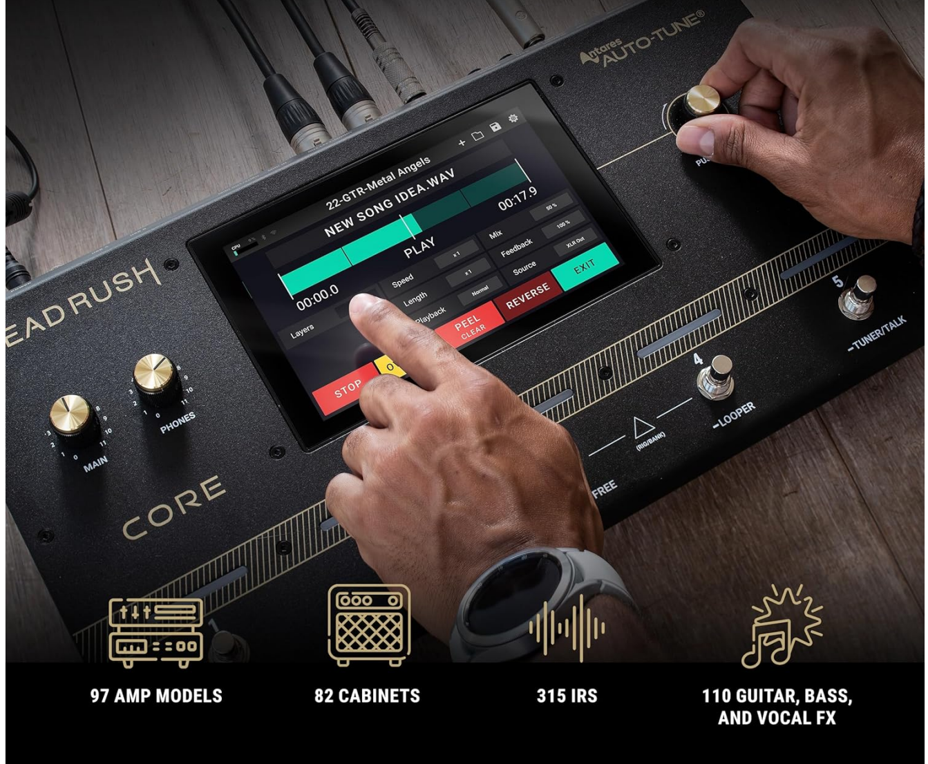
Figure 5: The 7-inch touchscreen interface for managing effects and rigs.
