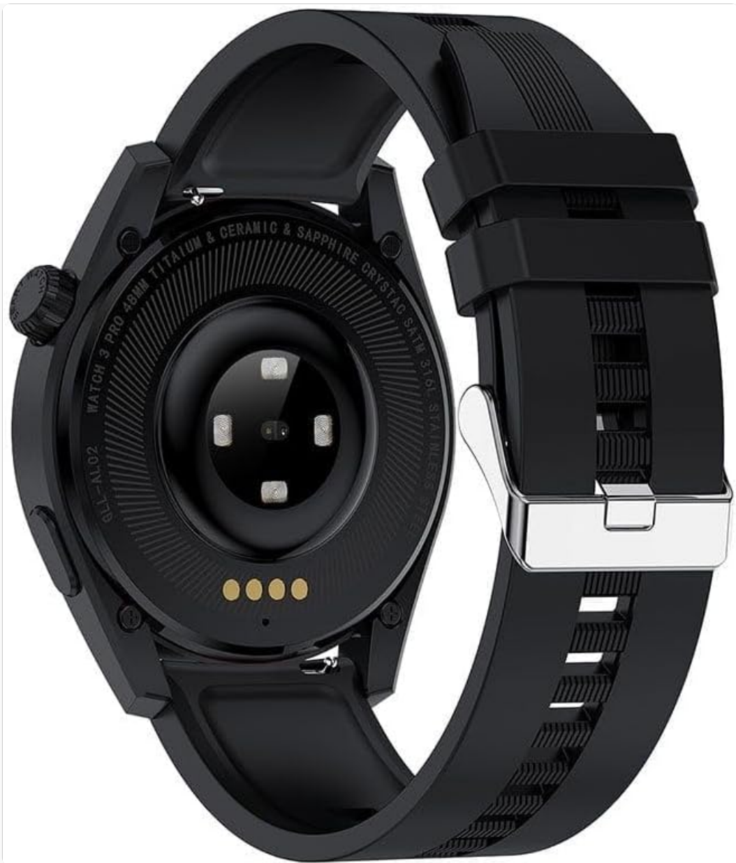
Figure 2.2: Rear view of the Devia Watch Pro 5 Smartwatch. This image highlights the back of the watch, featuring the optical heart rate sensor in the center and four metallic charging contacts. The watch casing is black, and the strap is also black silicone.
