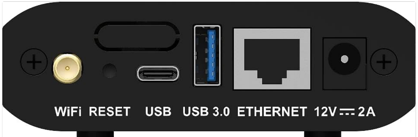
Figure 1: Side view of the LCB2K Media Player, showing audio, video, and communication ports.
