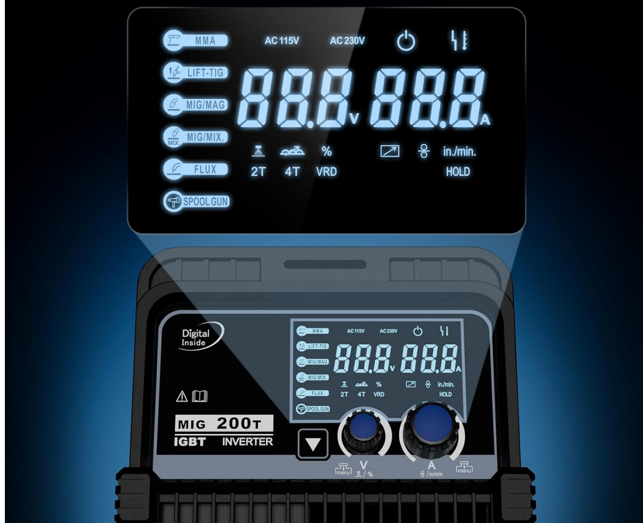
Figure 5: The synergic control display of the RILAND MIG200T, showing automatic parameter matching for various welding modes. Thanks to RICHIP technology, the machine offers true Synergic Control, automatically setting parameters once a process is selected. You primarily adjust the temperature (amperage/voltage) as needed.
