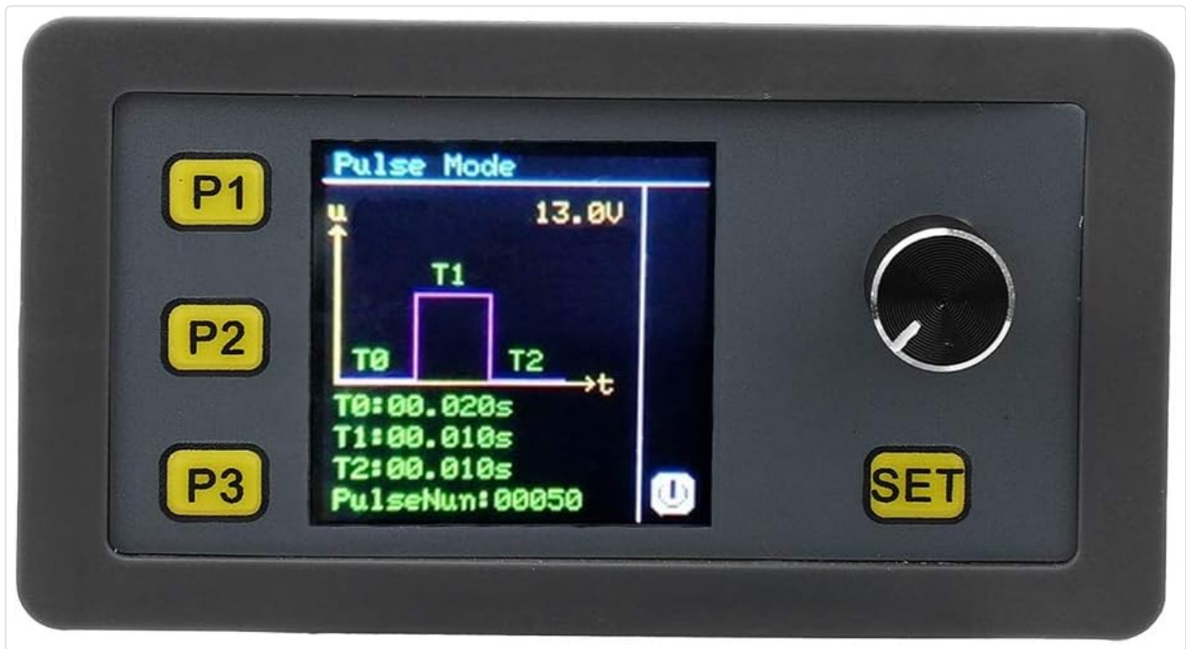
Figure 3.2: The module's display in Pulse Mode, showing adjustable parameters T0, T1, T2, and PulseNum, along with a graphical representation of the pulse waveform.
