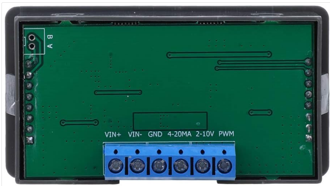
Figure 2.2: Rear view of the WSFG-06 module, displaying the screw terminal block for power input (VIN+, VIN-, GND) and signal outputs (4-20mA, 2-10V, PWM).
