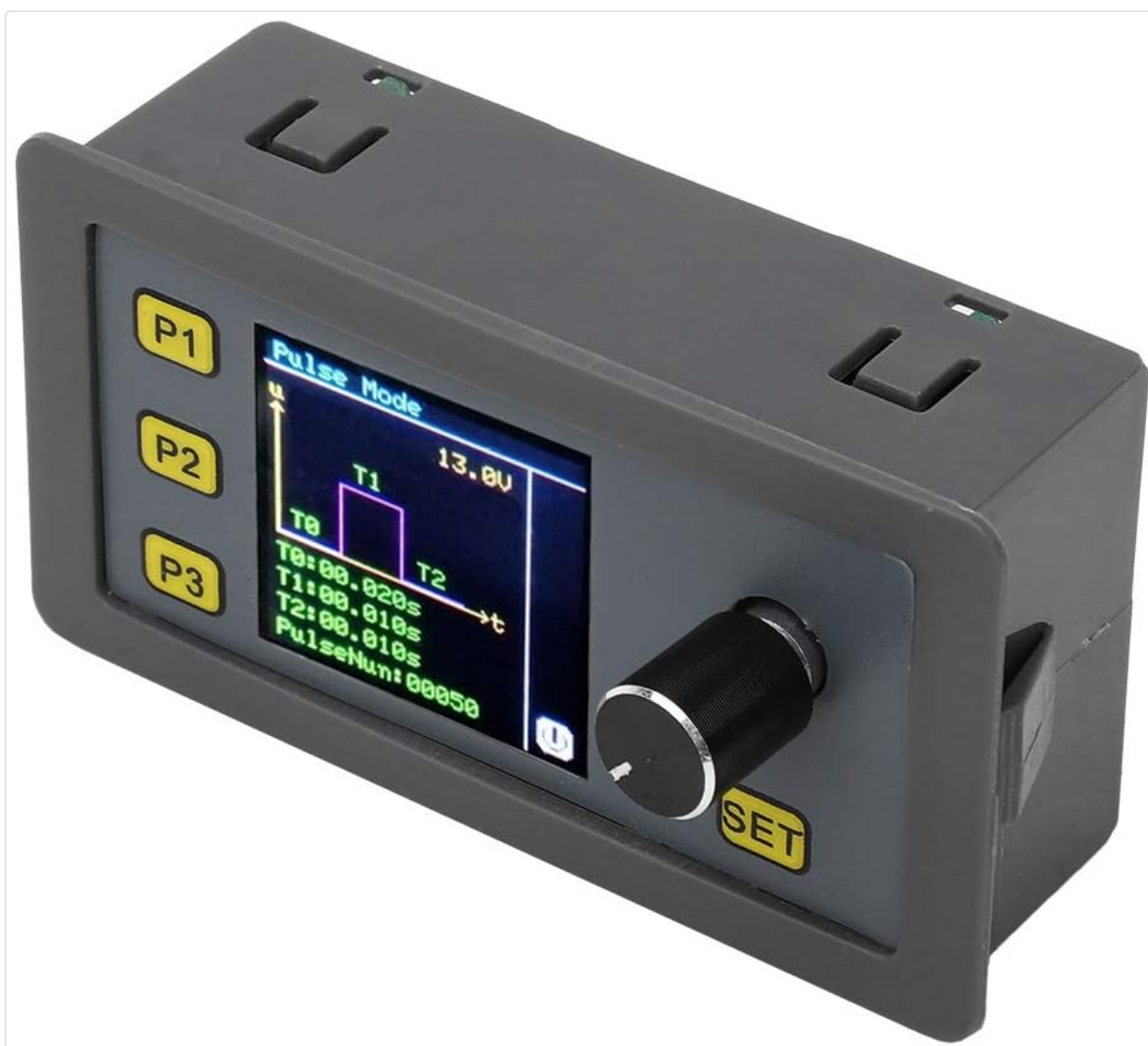
Figure 3.1: Front view of the WSFG-06 module, showing the display screen, rotary encoder (SET button), and programmable buttons (P1, P2, P3).
