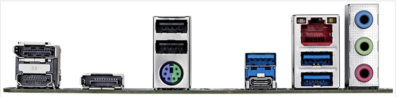
Image Description: A detailed view of the GIGABYTE B650M D3HP motherboard's rear I/O panel, showing various ports including USB, HDMI, DisplayPort, 2.5GbE LAN, and audio jacks.
