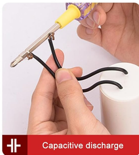
Figure 4.2: Illustrations of AC current, DC current, capacitive discharge, and capacitance measurements using the multimeter function.
