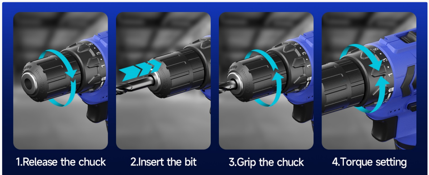
Image: Step-by-step guide for installing and setting up a drill bit.
