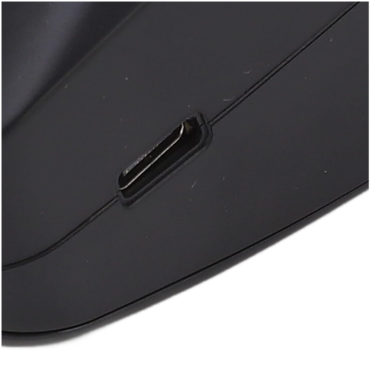
Image 2.2: A close-up view of the USB port located on the side of the printer, used for charging and data connection.
