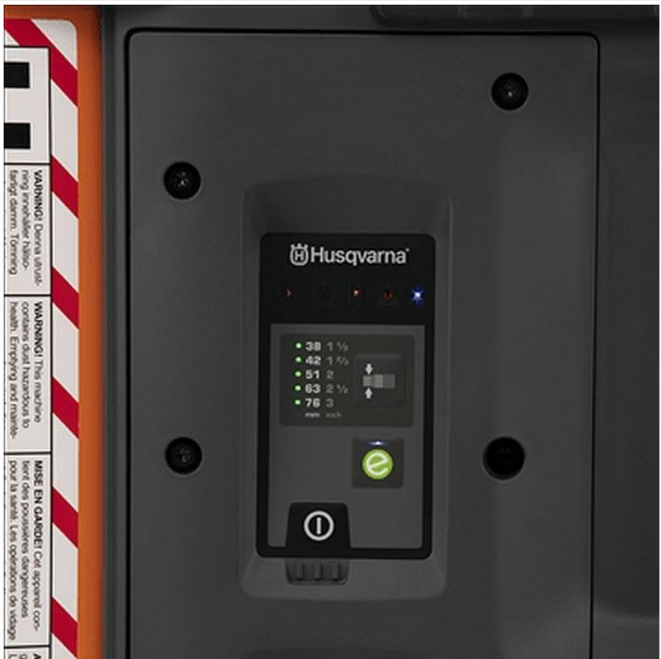
Figure 4: Detailed view of the HMI on the Husqvarna DE 120, showing filter status indicators and control buttons.
