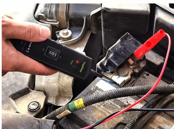
Figure 3: Proper connection of the Topdiag P55 to a vehicle battery and indication lights.
