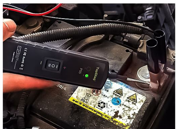
Figure 3: Proper connection of the Topdiag P55 to a vehicle battery and indication lights.
