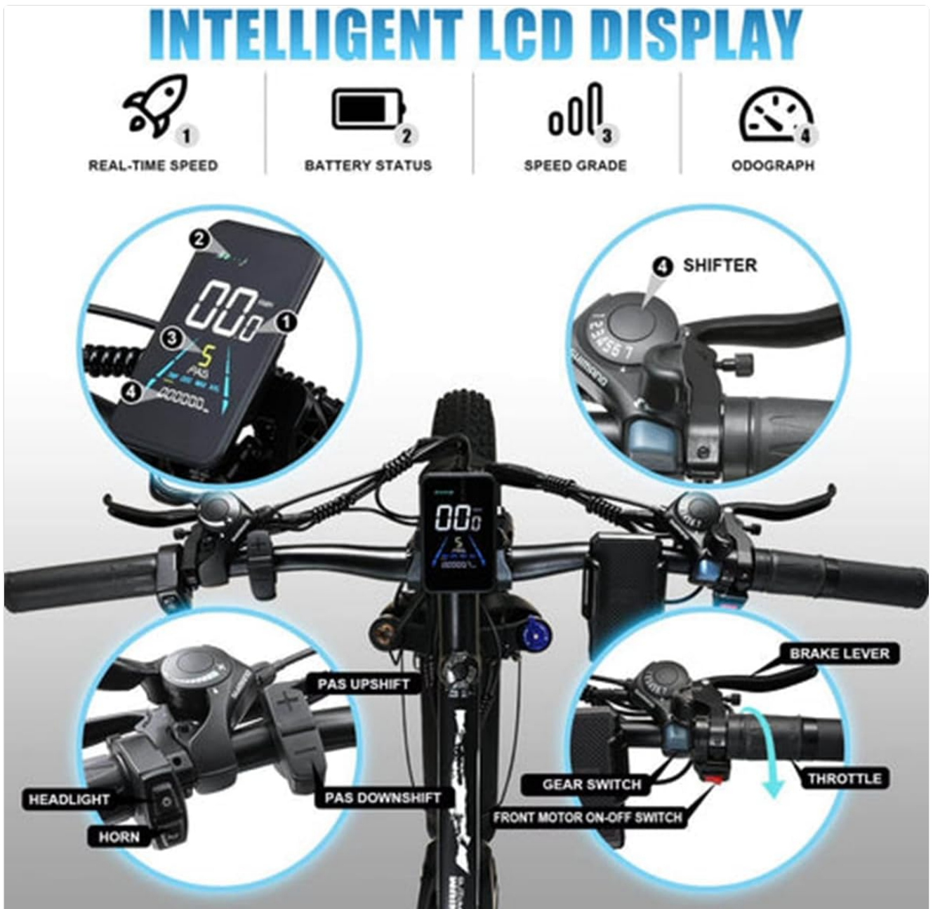
Figure 6: Overview of the intelligent LCD display and handlebar controls, including shifter, brake lever, throttle, headlight, horn, and motor switches.
