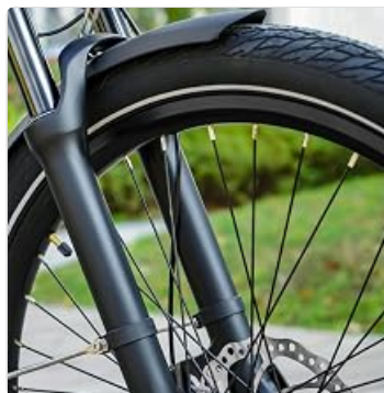
Figure 5.8: Front suspension fork for absorbing shocks.
