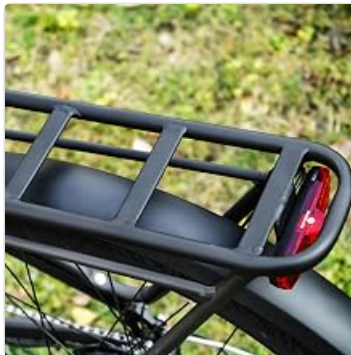
Figure 5.6: Rear rack with integrated tail light.
