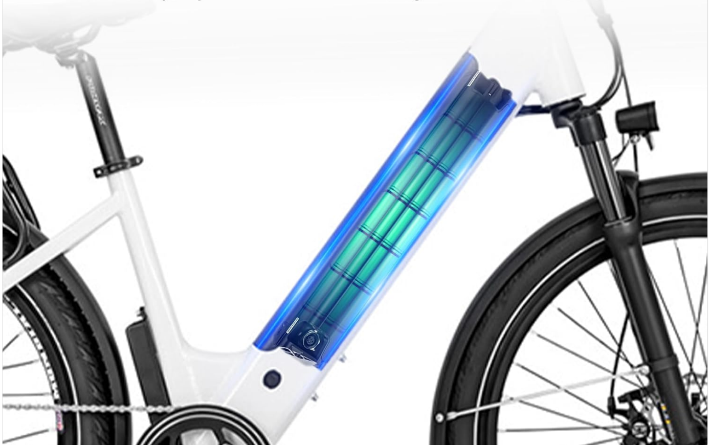
Figure 5.2: The removable 48V 16Ah battery integrated into the bike frame.
