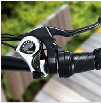
Figure 5.4: Shimano 7-speed shifter on the handlebar.
