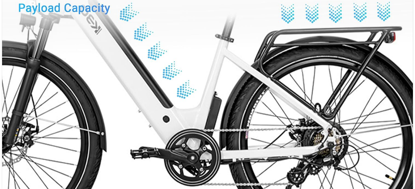
Figure 5.7: The robust 6061 aluminum frame design.
