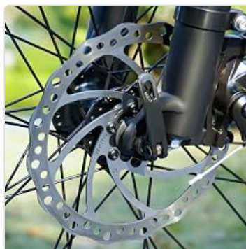
Figure 5.3: Close-up view of the disc brake system.
