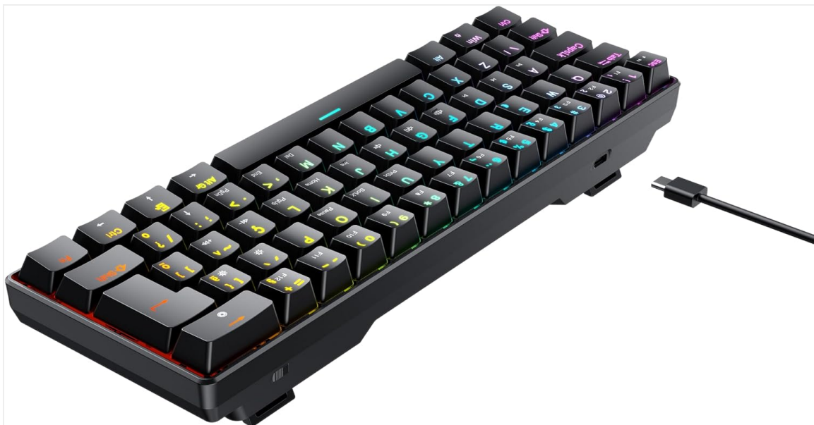
Image: Angled view of the Hyrax Thunder HCK61 Mechanical Keyboard, highlighting the detachable USB-C cable connection point.
