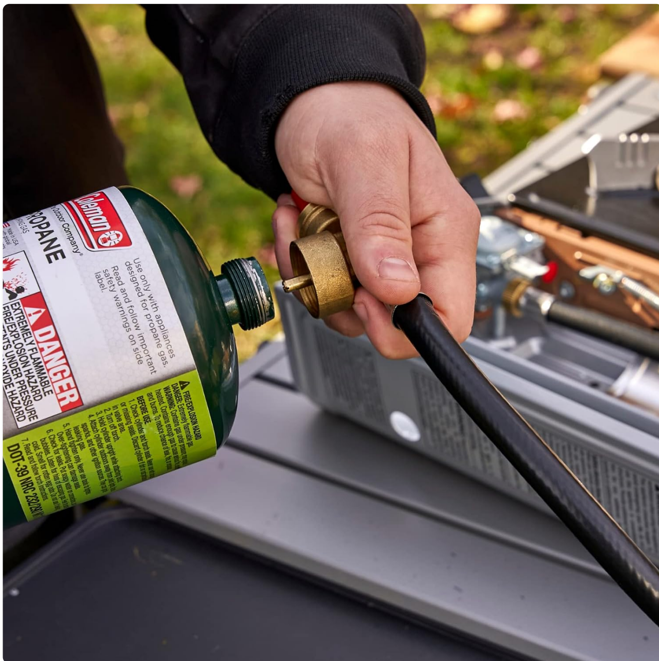
Figure 3: Demonstrates connecting a propane tank to the stove using the adapter hose.
