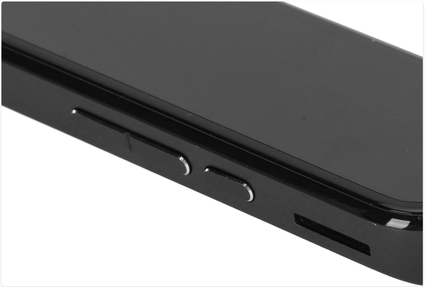
Image 5.2: Detail of the power and volume control buttons on the side of the device.
