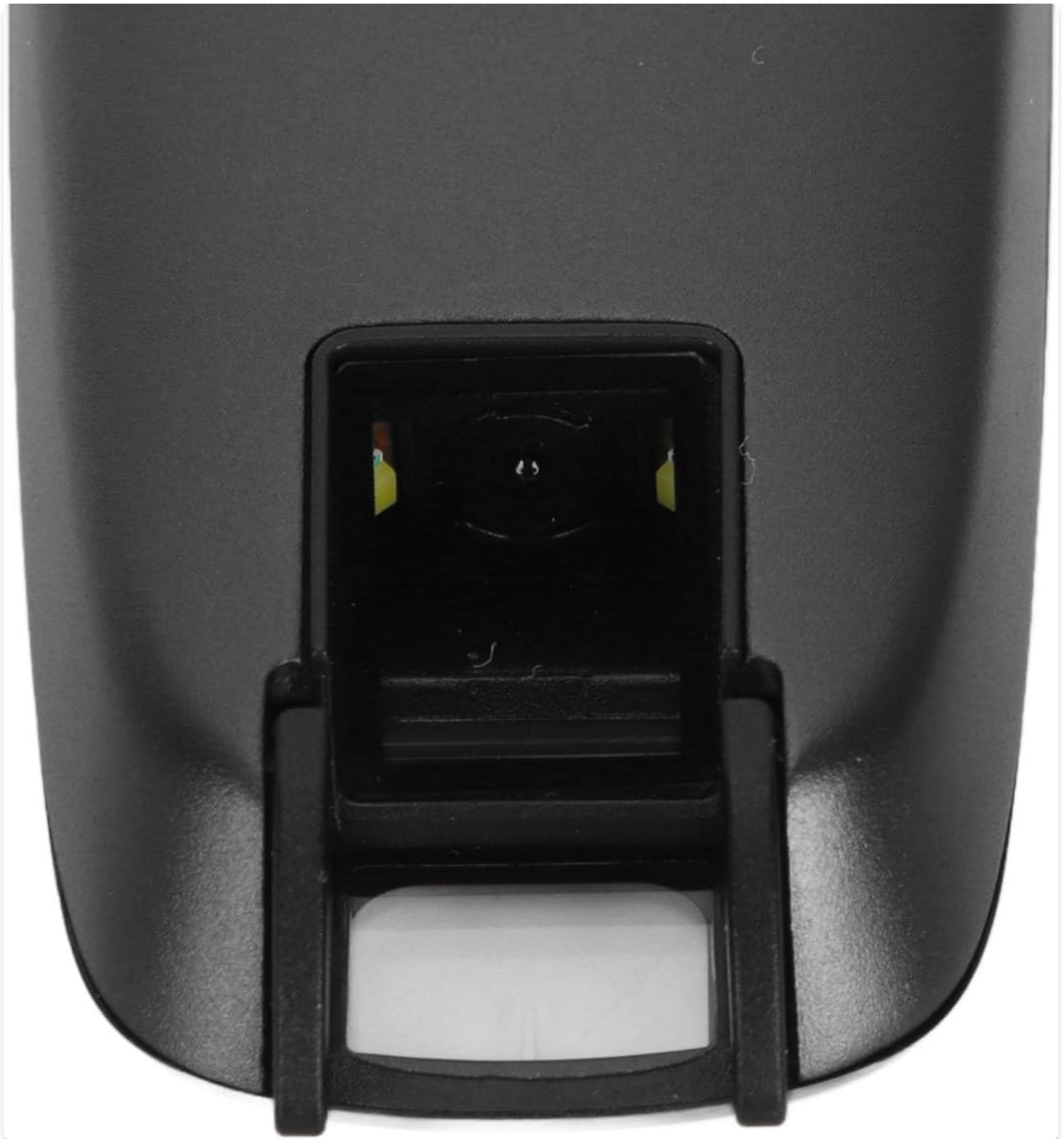
Image 6.3: Detailed view of the scanning head, which captures text for OCR and translation.
