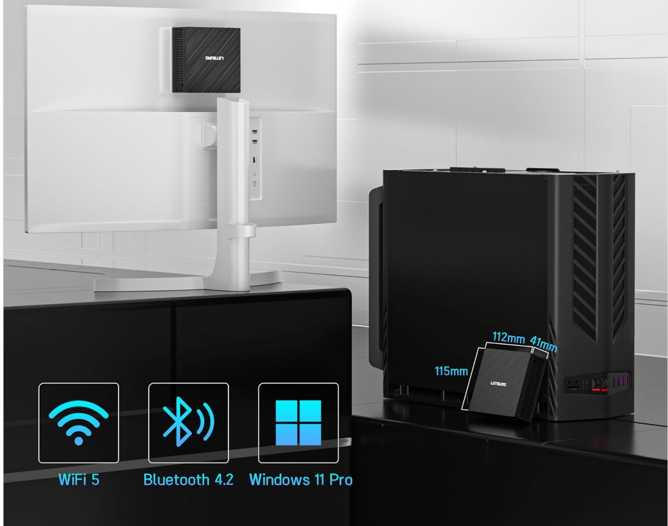
Figure 3.3: The Mini Air11 SE's compact dimensions and VESA mount capability.
