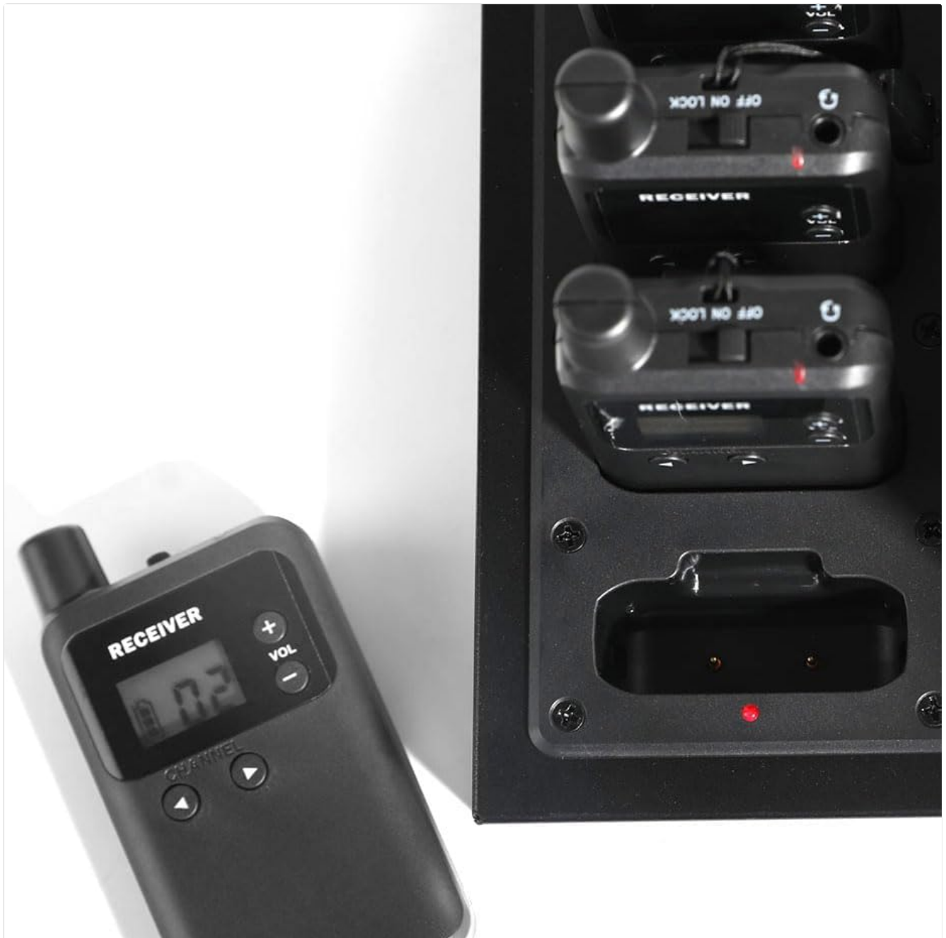
Image: A receiver placed in the charging station, indicating charging status with a red light.
