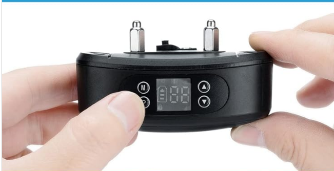
2.Long press the P button to open the device and start positioning.
