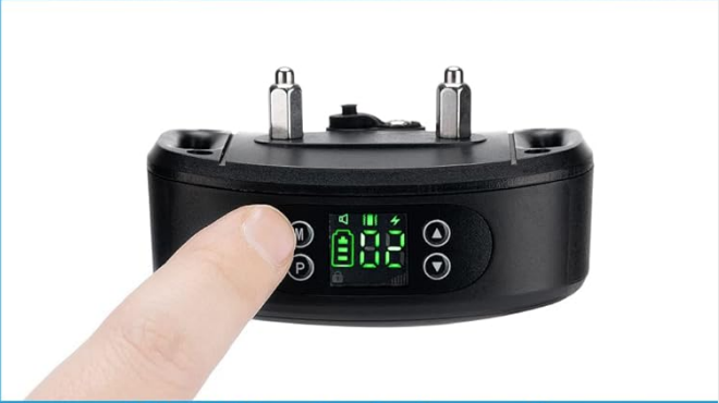
4.After finish setting the distance, short press M button to set the warning mode.
