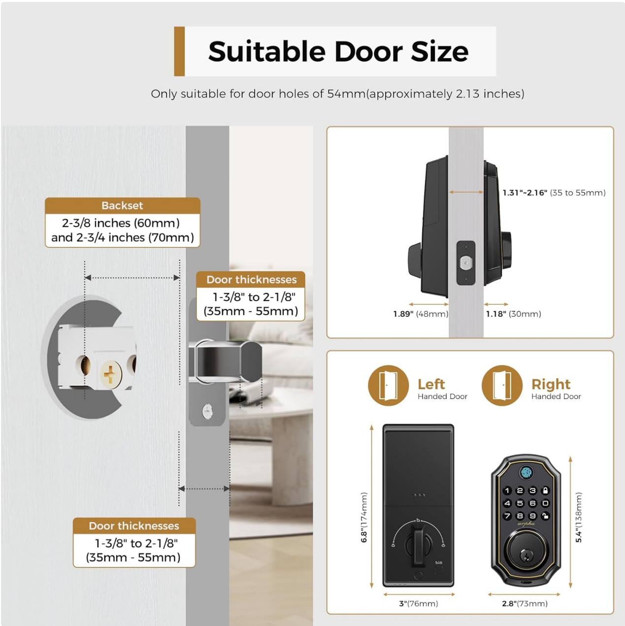
Figure 2.1: Door compatibility and dimensions for installation.
