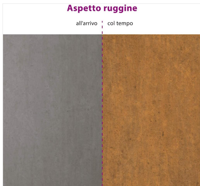
Image: Visual comparison showing the initial grey appearance of Corten steel upon arrival and its transformation to a rich rust color over time.
