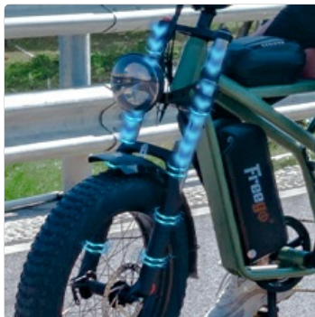
Figure 5.5: Detail of the front fork suspension, designed to absorb shocks and provide a comfortable ride.
