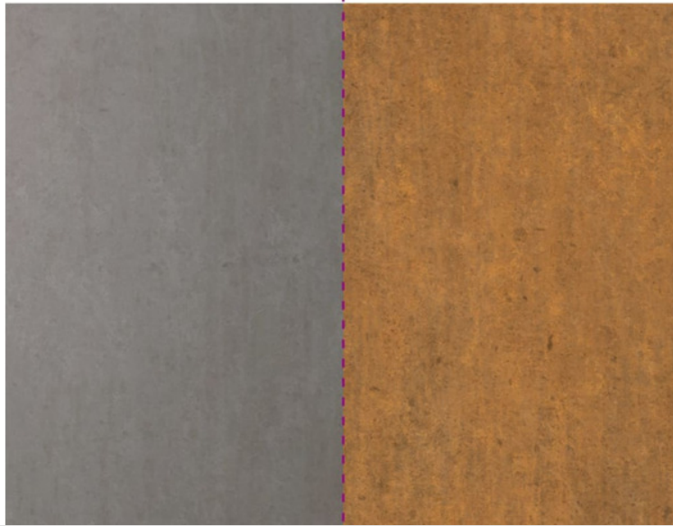
Image 5.3: Visual comparison illustrating the change in appearance of Corten steel from its initial state to its weathered, rusted state.
