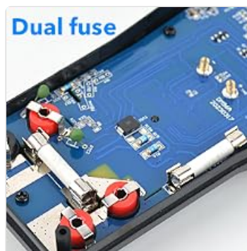
Figure 3.1: Dual fuse protection for enhanced safety.
