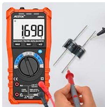
Figure 5.6: Diode test in progress.
