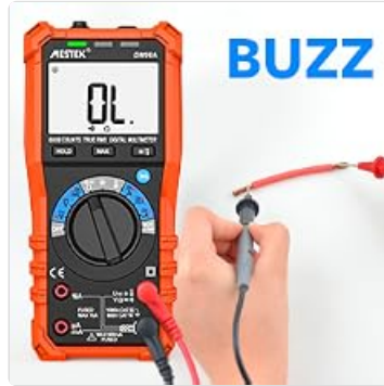
Figure 5.7: Continuity test with audible alert.
