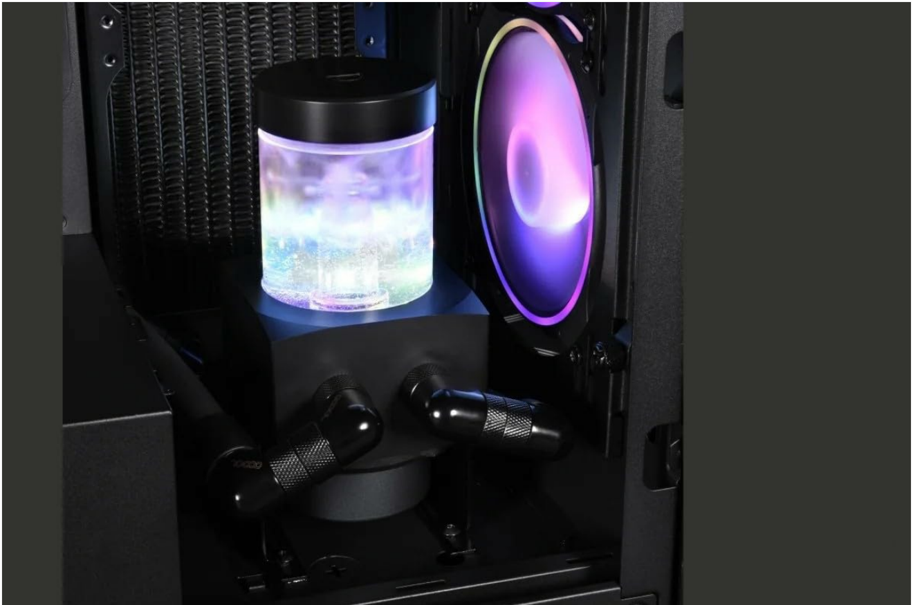
Image 4.1: The reservoir unit shown mounted on a radiator, demonstrating one of the installation possibilities.
