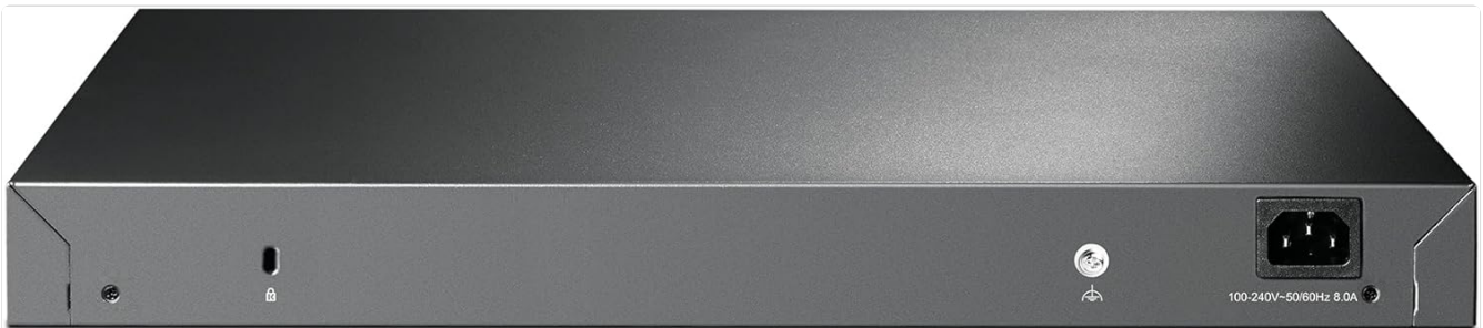
Figure 3.3: Rear view of the switch, showing the power input, grounding screw, and Kensington lock slot.
