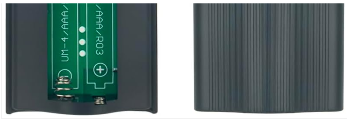
Figure 2: View of the open battery compartment showing the correct orientation for AAA batteries.
