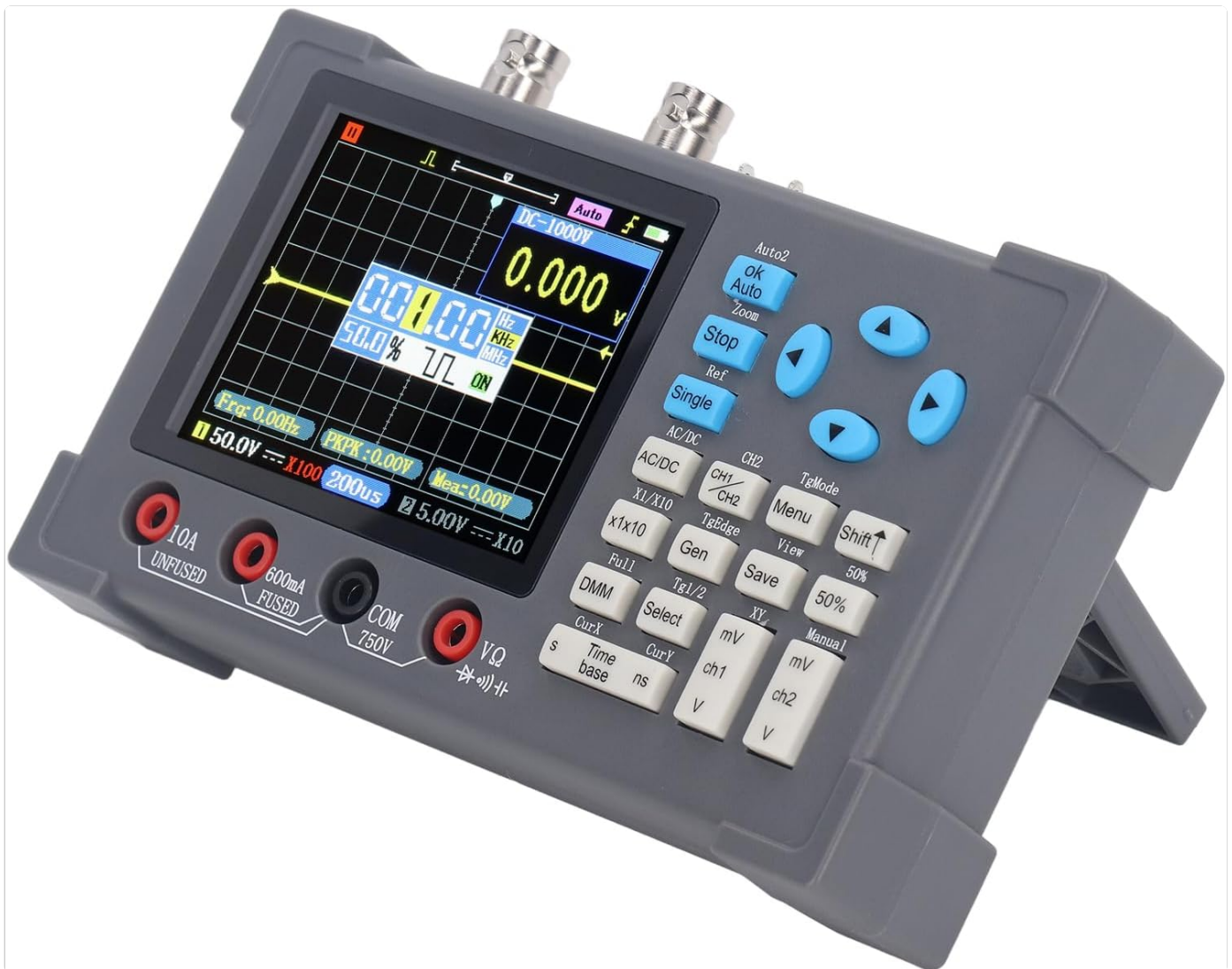
Figure 3.1: Front view of the DSO3D12, showing the display, control buttons, and input terminals.
