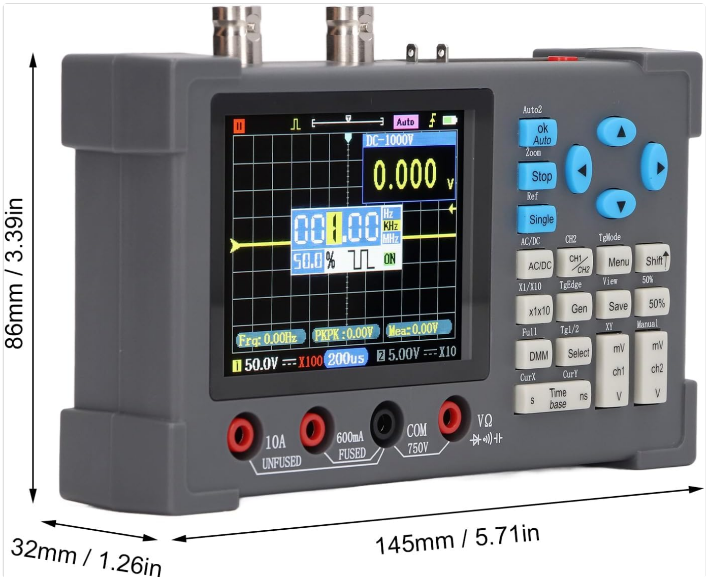
Figure 3.2: Dimensions of the DSO3D12, illustrating its compact size for portability.
