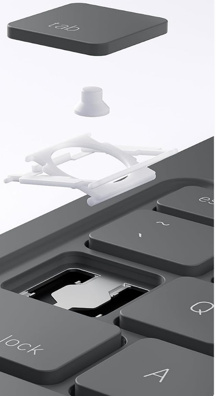
Figure 8: An exploded view of a key, illustrating the design elements that contribute to the ultimate typing experience, including keycap dimensions, key travel, and amplitude.
