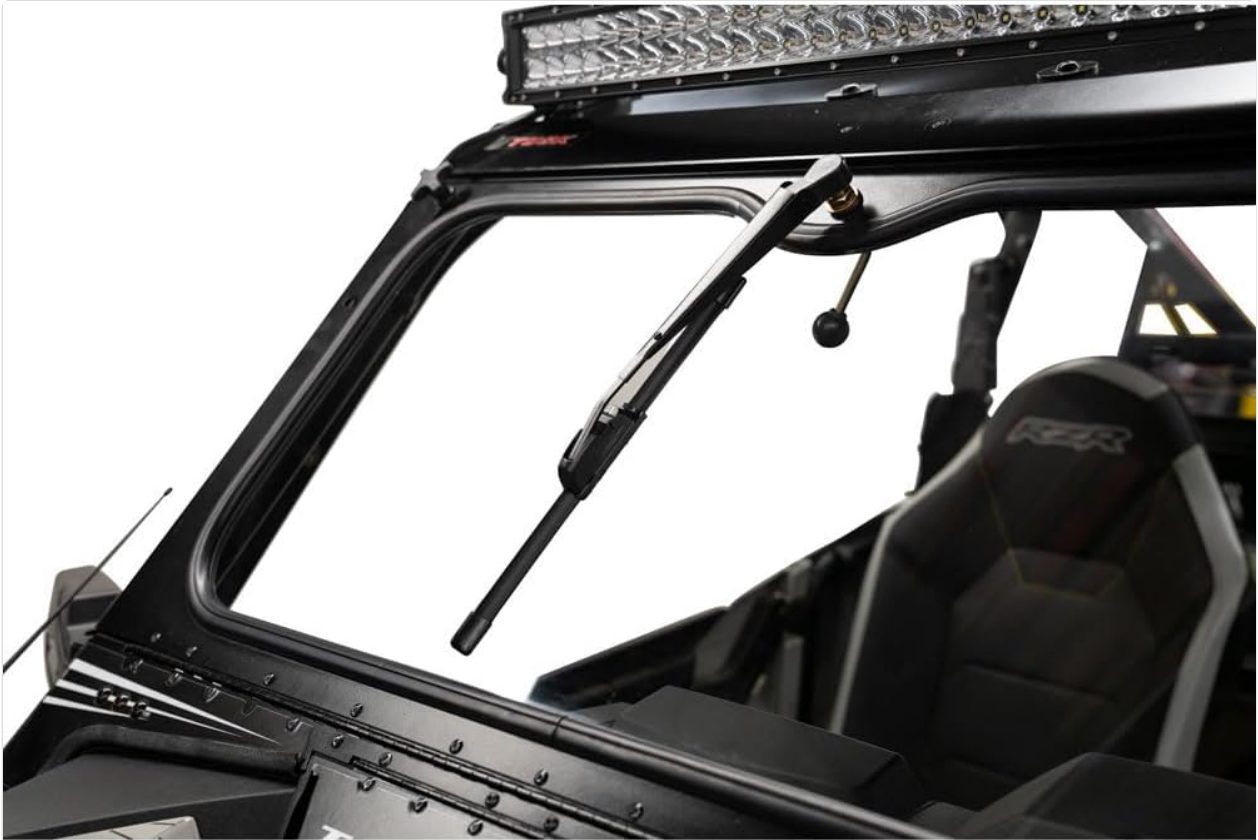
Image: A close-up view of the manual windshield wiper mechanism.
